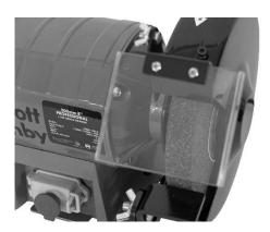
Position the eye shield so it does not come into contact with the grinding wheel. Using the wing nut (D) and 1 x washer (B), secure the eyeshield to the bench grinder allowing no more than a 2mm gap between the grinding wheel and bracket (A).
