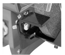
Attach the tool rest (A) to the bracket (B) using the long fastener (G) and the large washer (C) and wing nut (D). Then, attach this to the bench grinder using the 2 x small washers (E) and 2 x short fasteners (F), allowing no more than a 2mm gap between the grinding wheel and tool rest (A).
